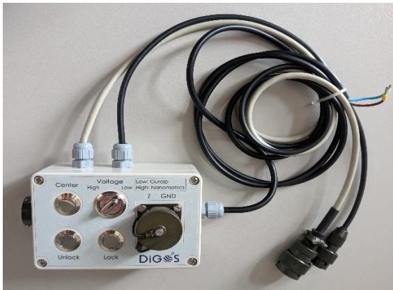
Photo of an example BOB with special functions (Un-Lock, Center...) and a schematic diagram to clarify individual customer requirements
