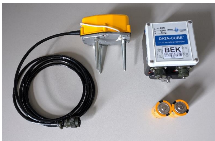
All components for DATA-CUBE 3 (Type 1) and Geophone installation
