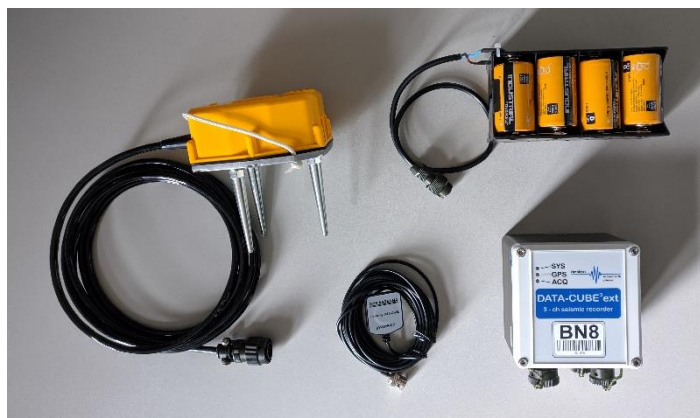
All components for DATA-CUBE 3 (Type 2) and Geophone installation
